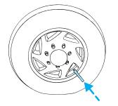
Periodically inspect the tire treads and remove stones, nails, glass or other objects that may be wedged in the tread grooves. Check for holes or cuts that may permit air leakage from the tire and make necessary repairs.
